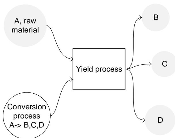
Figure 3-2: The dataset describing the processing of an input A into the products B, C and D is modelled as an independent processing activity simply providing the service of converting the input. With this approach the products B, C and D will be outputs of a
